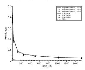
Fig. 2 RMSEs of signals against number of snapshots for fixed D = 1
